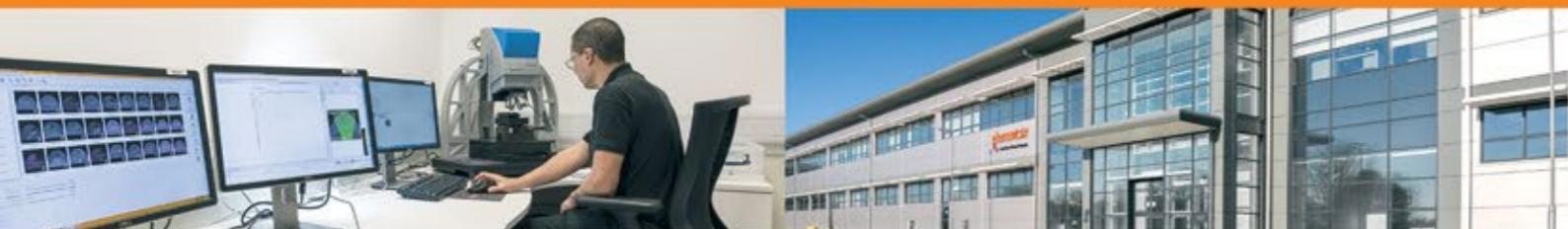
Andy Baker, Precision Test Operator at Element Six, uses Alicona on a daily basis for the measurement of insert geometries or tested tools.
