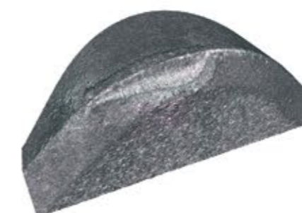
3D measurement of a cutting tool insert in true colour. Element Six compares the 3D structure of the tools before and after their usage to determine important parameters, such as the total volume of worn and accumulated material.
