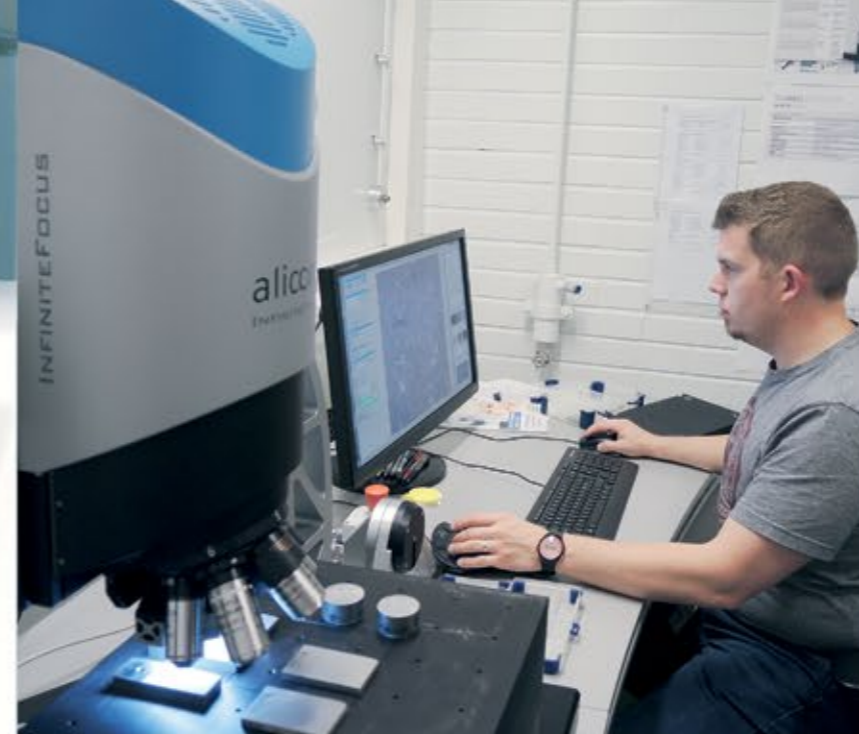
Niko Ojala, researcher at the Laboratory of Materials Science at TUT; using MultiMeasurement: With InfiniteFocus G5 Ojala defines the measuring routine with which several specimens are automatically measured one after another.
