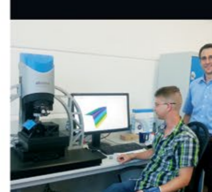
The 3D data sets of die and stamp are automatically superimposed. The resulting clearance is actually visualized by color coding and can also be accessed numerically at all points.
