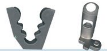
3D visualization of a turbine disc fir-tree root. Deviations from nominal geometries are automatically measured so that out-of-tolerance features are quickly assessed. 3D visualization of an injector combustion chamber. The optical measurement system by Alicona is used to verify geometry, positioning and functional dimensions.
