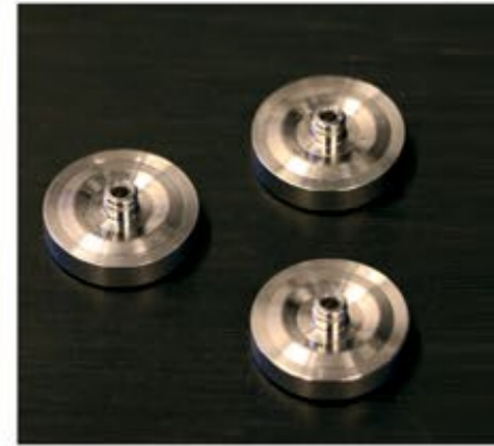
Using Alicona, Kendrion is able to measure the roundness of valve seats in a repeatable and traceable manner for optimal sealing.
